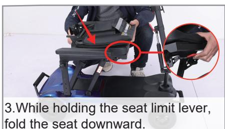
3. While holding the seat limit lever, fold the seat downward.
