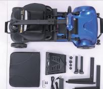
Take the scooter and the required mounting accessories out of the package
