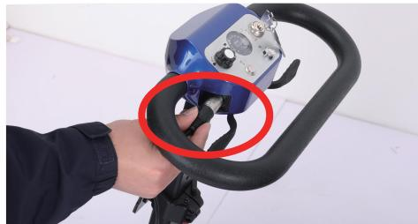
On the left side of the front of the scooter, there is a charging port. Use the standard charger to charge the scooter.
