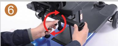
Adjust the armrest mounting seat to the appropriate position, then tighten the long handle screw. (Repeat this operation on the other side)
