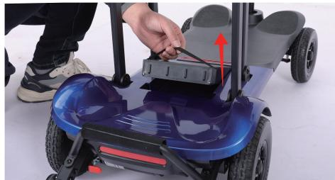
Grasp the battery handle and lift the battery upwards to remove it.
