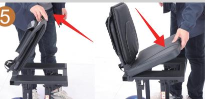
Unfold the backrest, then place the seat cushion on the seat frame
