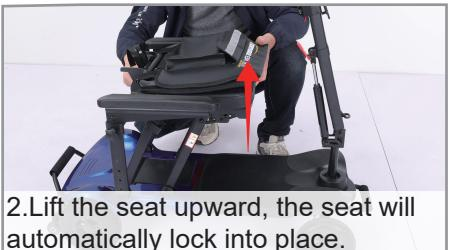
2. Lift the seat upward, the seat will automatically lock into place.
