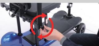
Adjust the armrest to the desired height, then tighten the long handle screw.(Repeat this operation on the other side)
