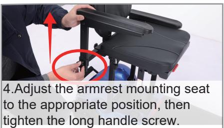
4. Adjust the armrest mounting seat to the appropriate position, then tighten the long handle screw.
